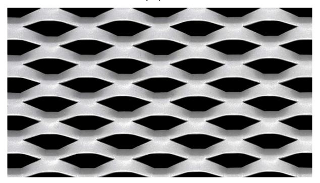
LW Pitch:38.10mmStrand Width:7.00mmSW Pitch:20.00mmThickness:1.20mmWeight:6.59 kg / m2Open Area:30%
